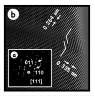
High-resolution images of sintered  $\mathrm{SnO}_2$  samples annealed under an oxygen atmosphere show structural defects that seem to be related to changes in both the cathodoluminescence spectra and electrical resistivity.
